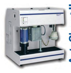
**The AutoChem II** performs a full array of highly precise, temperature-programmed studies. It uses the dynamic (flowing gas) technique to perform pulse chemisorption and temperature-programmed methods – reduction (TPR), desorption (TPD), oxidation (TPO), and reactions (TPSR) – as well as BET surface area evaluation.
