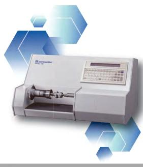
The GeoPyc utilizes a quasi-fluid displacement medium composed of non-hazardous microspheres having a high degree of flowability that do not wet the sample or fill its pores. Determines envelope volume and density of monolithic samples as well as the bulk volume and density of powdered materials wide range of sample sizes
