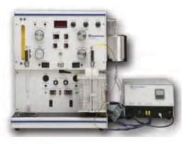
**ChemiSorb 2720** – Dual station, one for analysis and one for sample preparation
