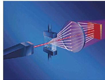
Static light scattering makes use of the **Mie theory** of light scattering by particles. Mie theory describes characteristics of the scattering pattern (light intensity versus scattering angle, among other things) produced by the interaction of a plane wavefront of monochromatic light with a spherical, isotropic particle suspended in a medium of known optical properties.
