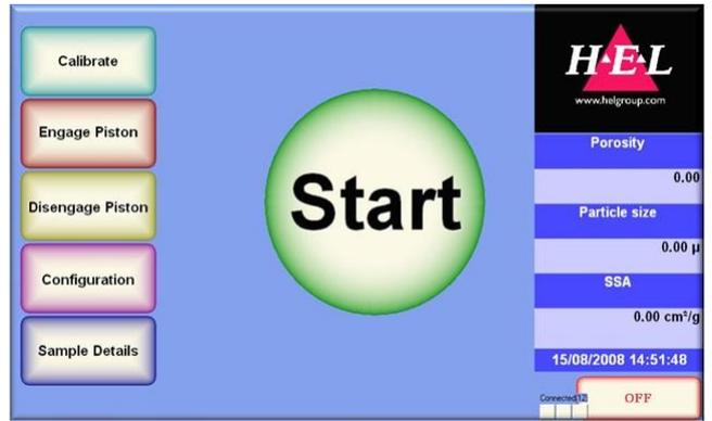
A touch screen interface makes operation and report generation simple, with the option to insert company logos and typestyles, and to use various formats when printing.
