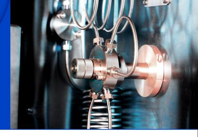
The MICROACTIVITY-Reference is an automatic and computerized laboratory reactor for reactions of catalytic microactivity with reactor bypass, preheater evaporator, pressure control valve and other process layouts in hot box, which avoids the possible condensation of volatile products, at the time that preheats the reactants efficiently.
